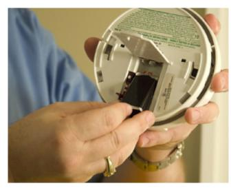
These batteries must be tested on a regular basis and, in most cases, should be replaced at least once each year (except for lithium batteries). See the Smoke Alarm Maintenance section for more information.
